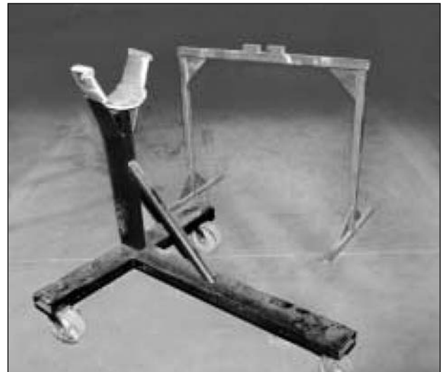
Illustration 1. Two examples of center tube end supports.
