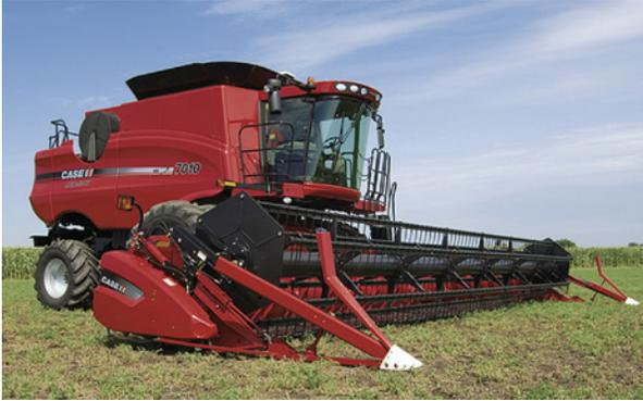
With staggered tines spaced 6 inches, HCC Reels provide a 3-inch effective tine path, moving crop more efficiently.
