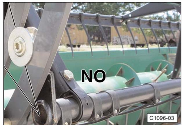
Incorrect orientation (roller is above or following the tine tube into header).
